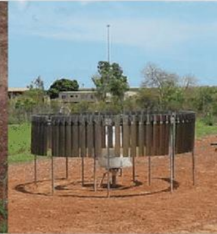
(b) Weighing bucket rain gauge
