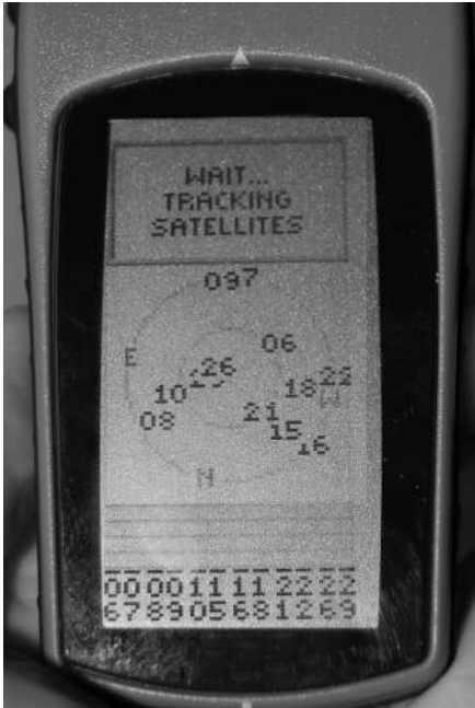
Figure 3-1. A common handheld GPS device used by geocachers to locate hidden geocaches
